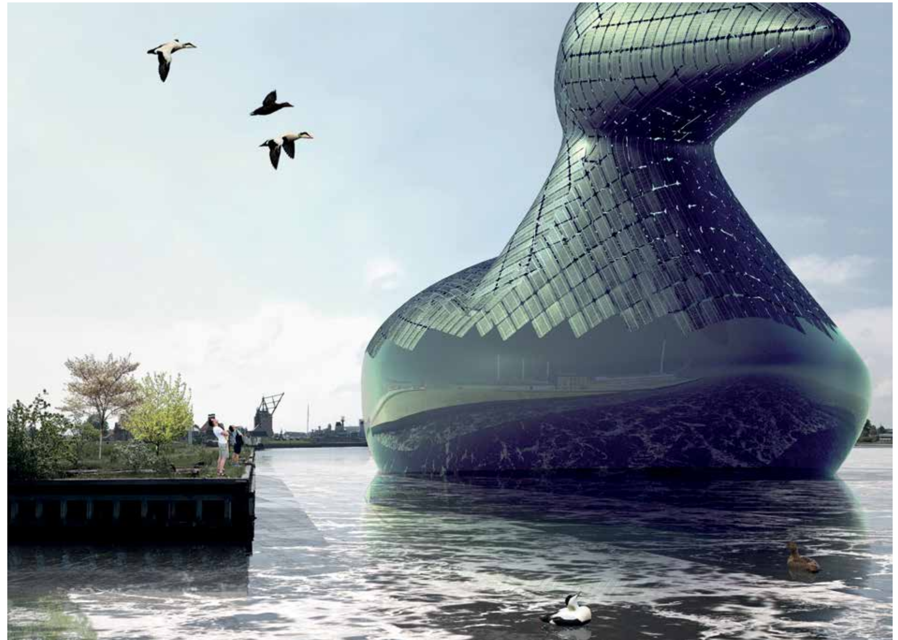
Energy Duck can be used to cover short-term fluctuations in available sunlight by allowing its hull to fill with water.
